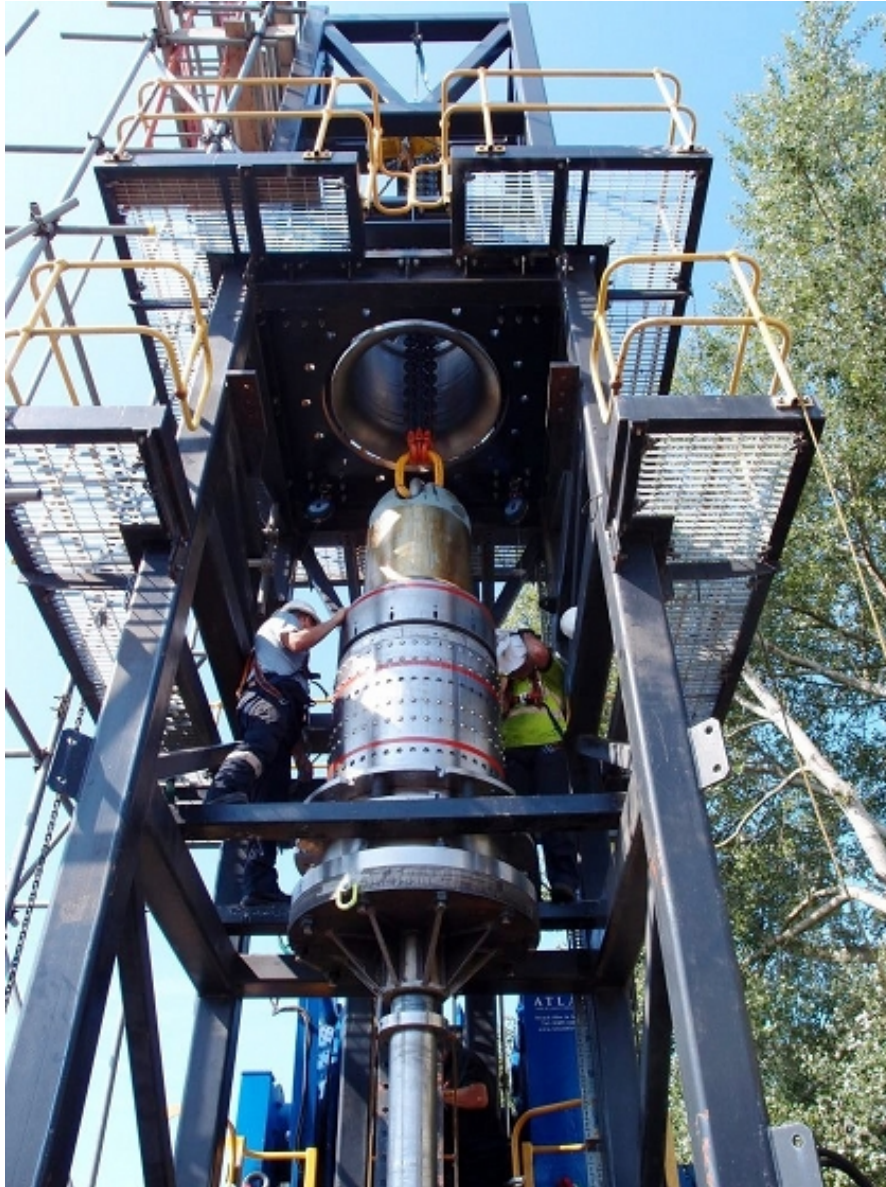
First Subsea bend stiffener connector undergoing testing on the company's dedicated test rig.
