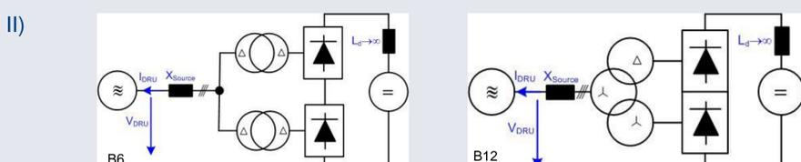
Finally, distributed WTG converter feed the considered rectifier bridge whereby the power is collected along one cable string. The used control concept relies on the fundamental frequency in the power system to establish uniform reactive power sharing between individual WTG converters via application of a common droop. An equivalent for the cable string is determined which requires less computational effort in large system studies.
