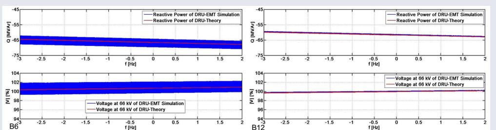
III) A system of 72 MW is investigated with detailed cable string model. Surprisingly, reactive power demand of B6 is smaller than B12. This occurs due to the high voltage distortion leading to harmonic interaction effects. Cable sections are replicated here with travelling wave model.
