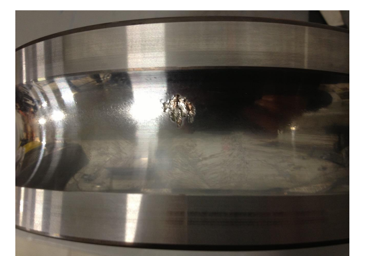
Example of Damaged Bearing
