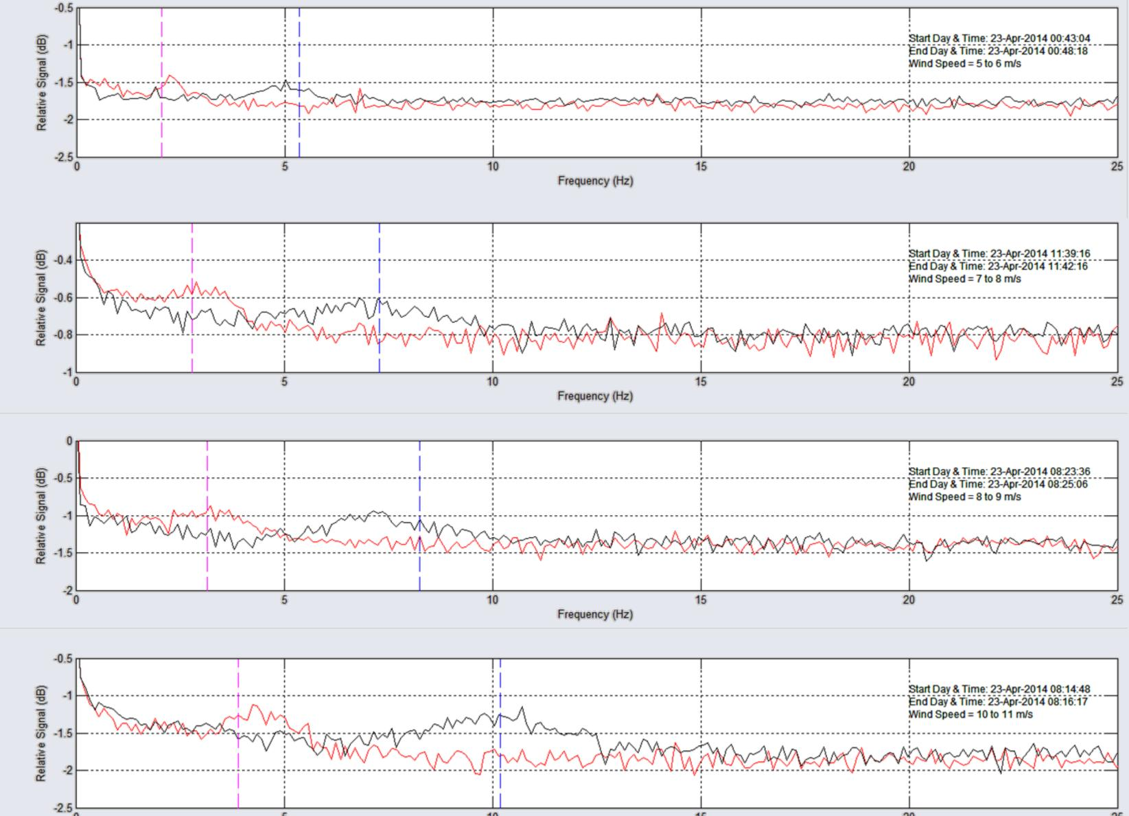
The frequency content of the fluctuations pressure was analyzed with an expected vortex shedding frequency predicted by the Strouhall relationship below. This frequency is a function of the Strouhall number, the trailing edge thickness of the blade, and the local wind speed.
