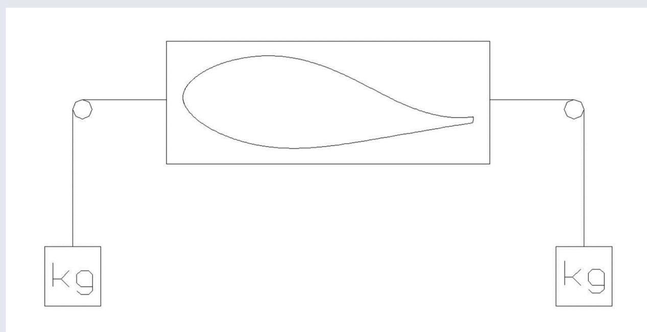
Consequently, it is possible to decrease the overload on much of the blade and at the same time reach the required bending moment at the root. This method will also permit a small increase in the general load level, whereas the overload it kept at an acceptable level. This increase will also permit a reduced number of load cycles. Assuming that the blade is made of polyester, an increase of loads by 7 % will reduce the number of cycles to 50 %.
