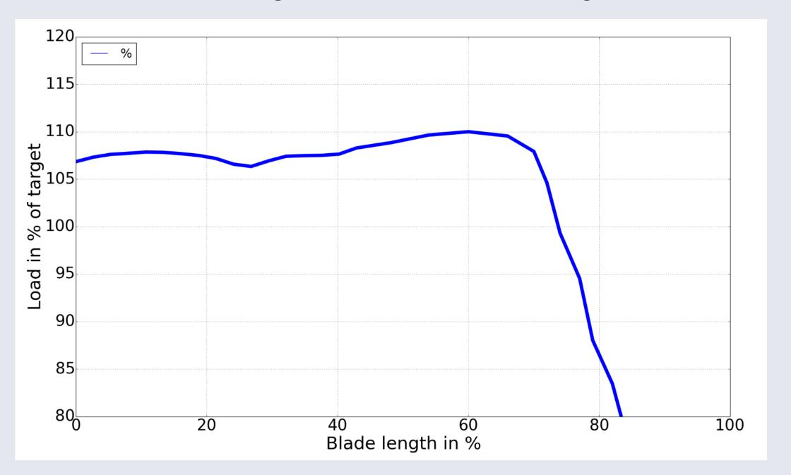
Furthermore, BLAEST has developed different oscillation amplifiers for both edgewise and flapwise directions which do not affect the blade unintendedly. Below figure shows an example for an edgewise horizontal test direction.
