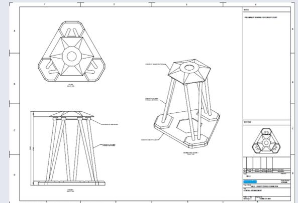
As a gravity structure the Gravity Tripod removes sub-seabed risk and the geometry, as well as mass distribution, of the design simplifies design of the nodal connections between components. Through modular design the Gravity Tripod minimises component manufacturing and assembly times as well as the space requirements for construction, making it suitable for manufacture at a wider range of locations than for other offshore wind sub-structures.
