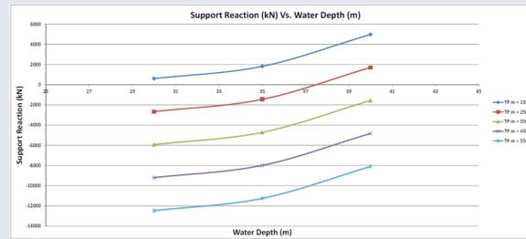
Two wave directions were found to be critical, the 000 degree and the 030 degree waves, all other combined load cases were excluded
