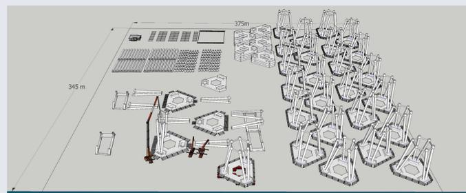
The Gravity Tripod is designed for rapid assembly. As a modular structure manufacturing of the components ahead of assembly limits the space and time required to supply a large number of structures.
