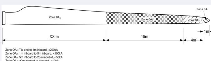
Figure 5. Zoning concept enabling direct attachment on the entire blade surface.
