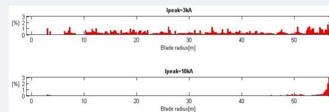
Figure 4. Attachment to the blade vs. the blade radius (60m blades). Comparison between the attachment simulation results for different  $I_{peak}=3, 10kA$ . For current larger than 10kA attachment is most likely within 5m from the tip (between 70-90% of the attachments), while currents around 3kA can attach along the entire length of the blade.
