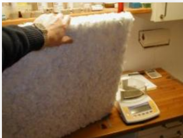
Figure 5 Insulation wool mat made out of blade fibre
