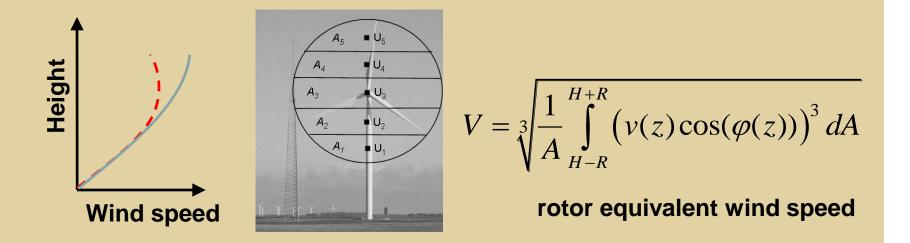
Tip-height measurements (using remote sensing devices e.g. LiDAR/SoDAR) have a big role to play in improving wind resource assessment.
