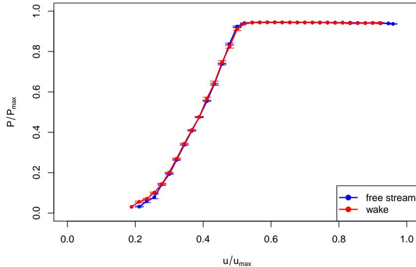
Figure 2: Langevin Power Curves (LPC) of a multi-MW offshore wind turbine. Wind speed was measured by a nacelle-based scanning lidar system [5]. Power performance is shown for free stream (blue line) and wake conditions (red line).
