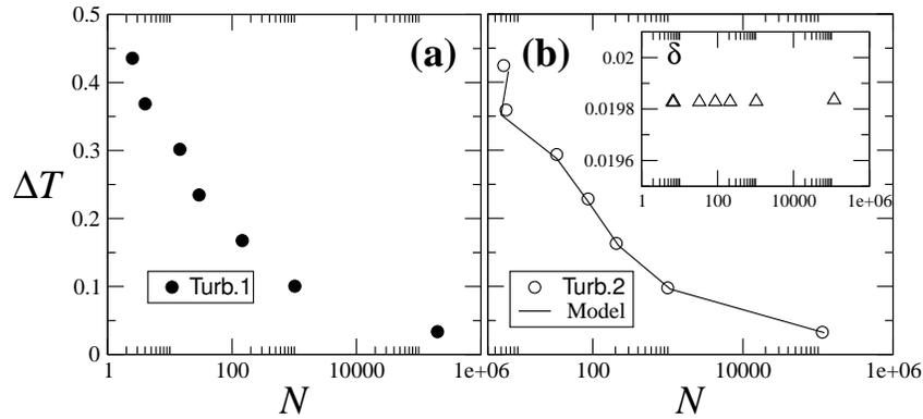
Figure 1: Torque statistics (rainflow counts) at the main shaft of two neighboring multi-MW turbines in the same offshore wind farm. (a) measured torque statistics at turbine 1, (b) torque statistics at turbine 2, both measured (symbols) and reconstructed (solid line) by the stochastic model (1). From turbine 2 only the wind speed time series of the nacelle anemometer was used.
