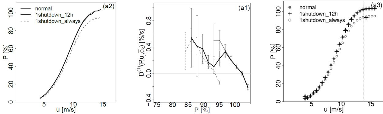
Figure 3: Wind farm performance monitoring by 10 minute averages as in IEC 61400 (left), by the drift coefficient  $D^{(1)}$  of eq. (1) (middle), and using the LPC (right). Line styles of the left graphic apply to the middle one as well, here showing clearly a transition between two power performance states. The measured cumulative power output of twelve turbines was used, where the contribution of one turbine was artificially set to zero for 12 h.
