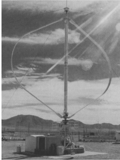
Figure 1: SNL 17m Darrieus vertical axis wind turbine [7].
