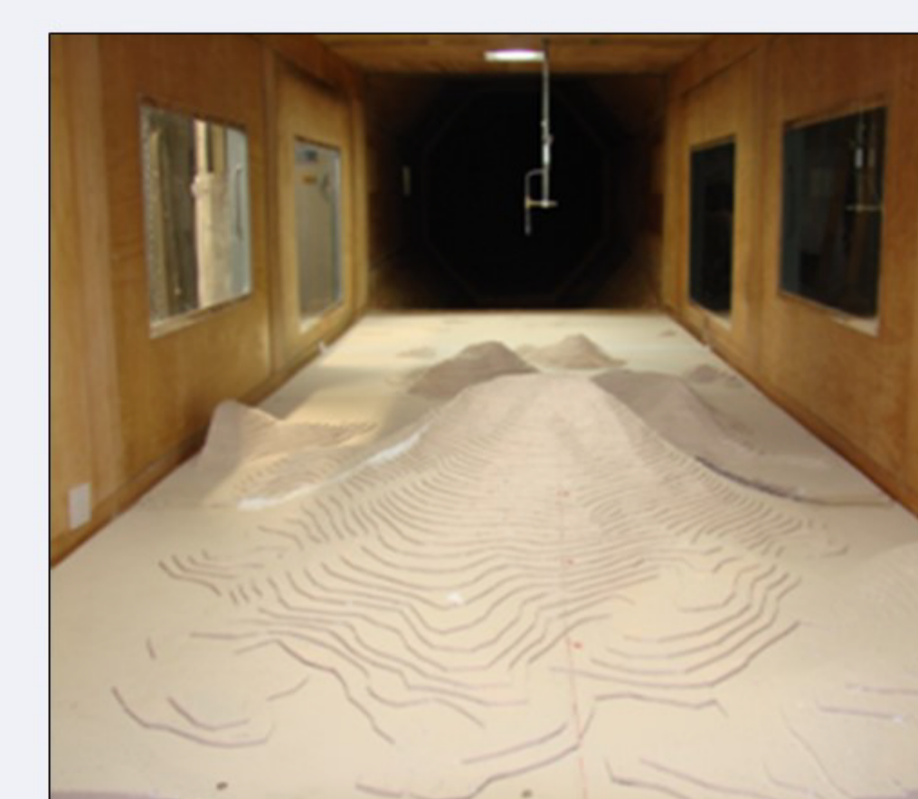
Fig 2. Model at the Boundary Layer Wind Tunnel
