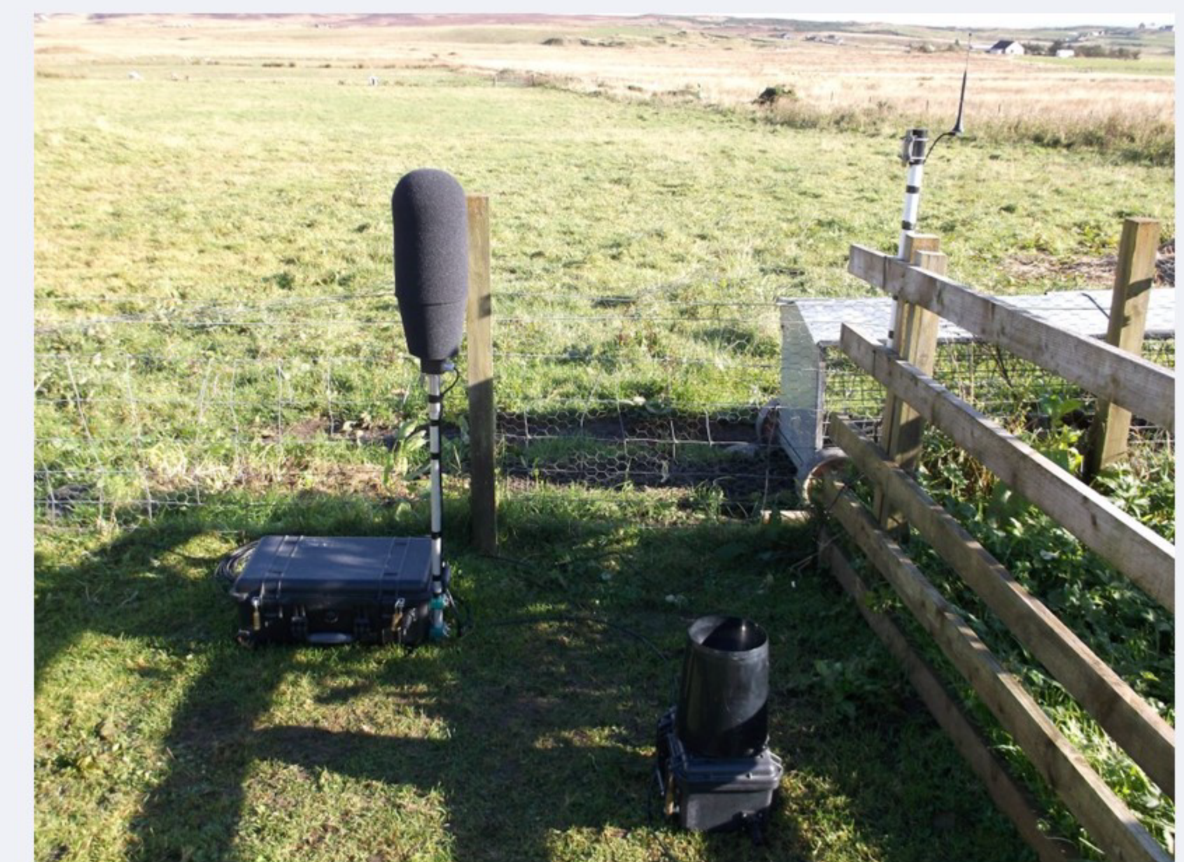
Example of a smart meter with in-situ data processing, including a rain gauge allowing exclusion of rain-affected periods
