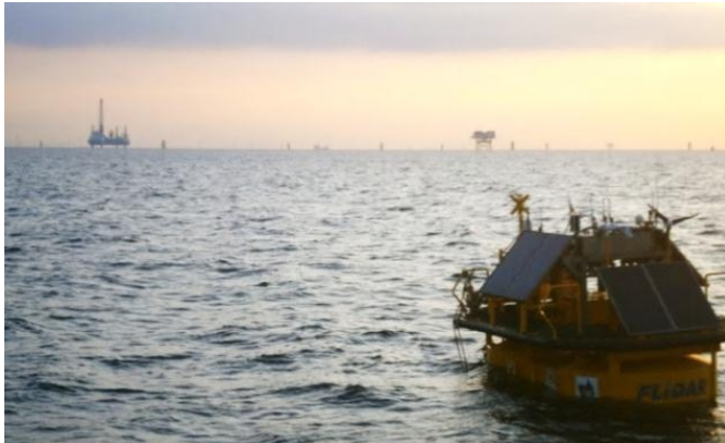
Fig. 1: A FLiDAR buoy measuring wind resource in the Irish Sea
