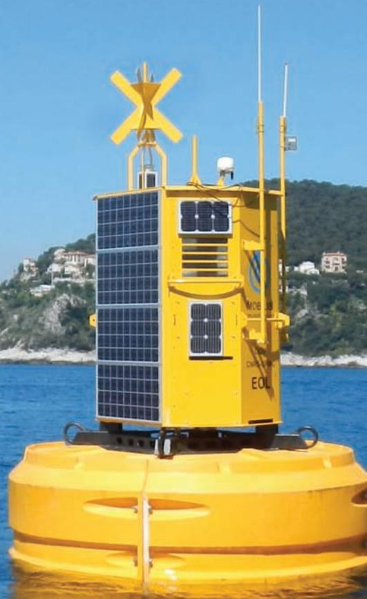
FLiDAR's floating Lidar system
