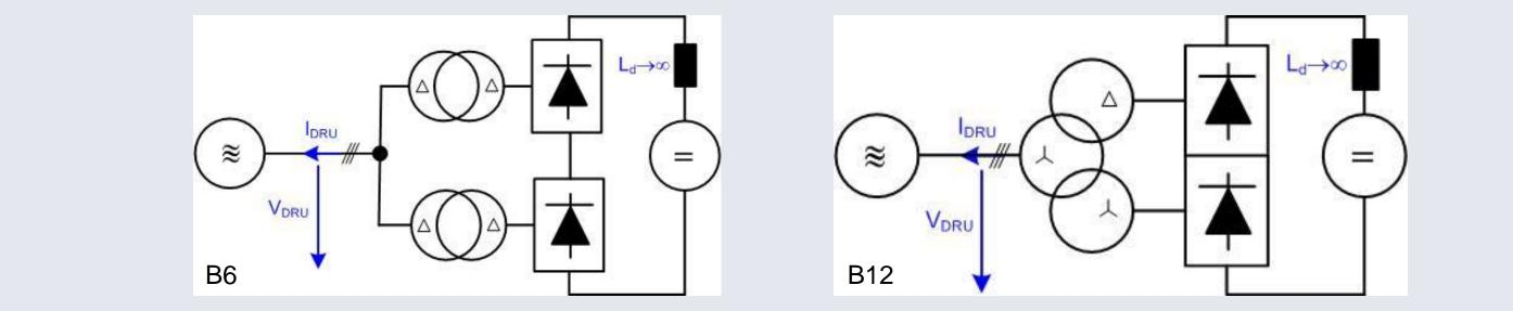
III) A system of 72 MW is investigated with detailed cable string model. Surprisingly, reactive power demand of B6 is smaller than B12. This occurs due to the high voltage distortion leading to harmonic interaction effects. Cable sections are replicated here with travelling wave model.
