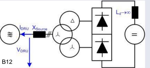
voltage distortion. This will reduce costs for reactive power compensation and cable losses in return for slightly higher costs of 12-pulse DRU equipment in comparison to 6-pulse equipment. Harmonic filter could also be significantly smaller.
