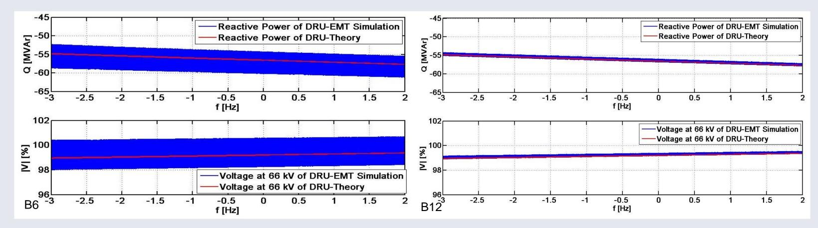
II) The analytical theory is now extended to a system with finite source reactance X<sub>Source</sub> by setting X:= $X_{Tr}$ + $X_{Source}$ ·(6/q) whereby q=6 for B6 and q=12 for B12.
