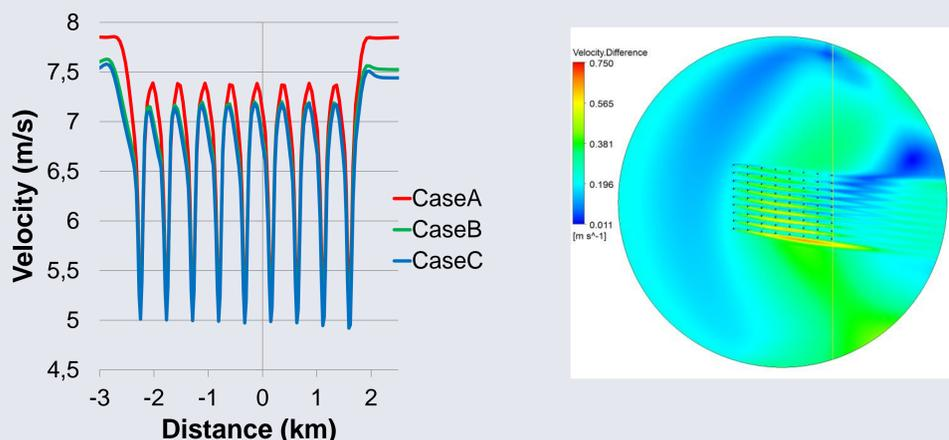
Figure 3: Left: Horizontal velocity one diameter downstream from the farm, across the yellow line in Figure 1. Right: Difference in wind speed velocity at hub height (CaseA minus CaseB).
