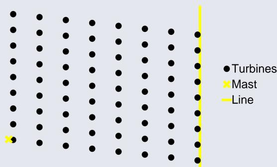
Figure 1: Locations of wind turbines (black dots), the upstream met mast (yellow cross) and wake measurement line (yellow line).
