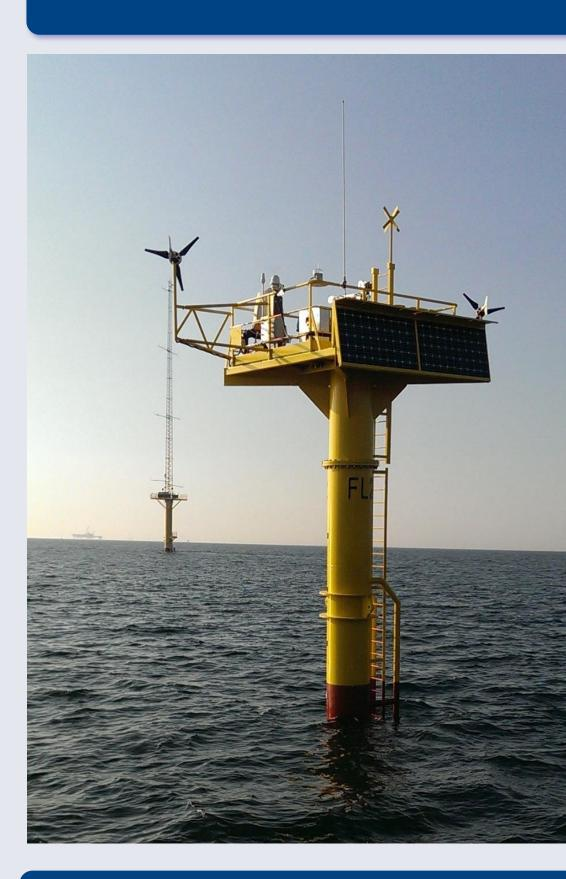
Babcock's FORECAST floating LiDAR system is based around a low motion, shallow draft spar buoy which is designed to minimise the wave, wind and tidal current induced pitch and roll.
