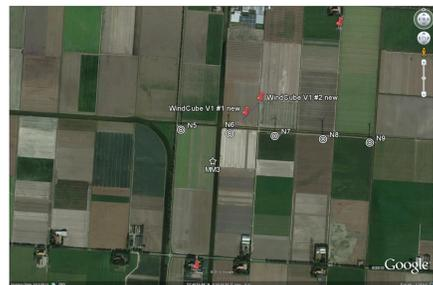
**Layout of the test site with turbines, mast and LiDARs indicated.**
