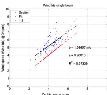
The nacelle LiDAR wind speed measurements are validated against the mast for strictly North-East winds. The Wind Iris measurement distance of 200m is used and for the Zephir the distance of 49m. The latter is the largest distance still inside the wake.
