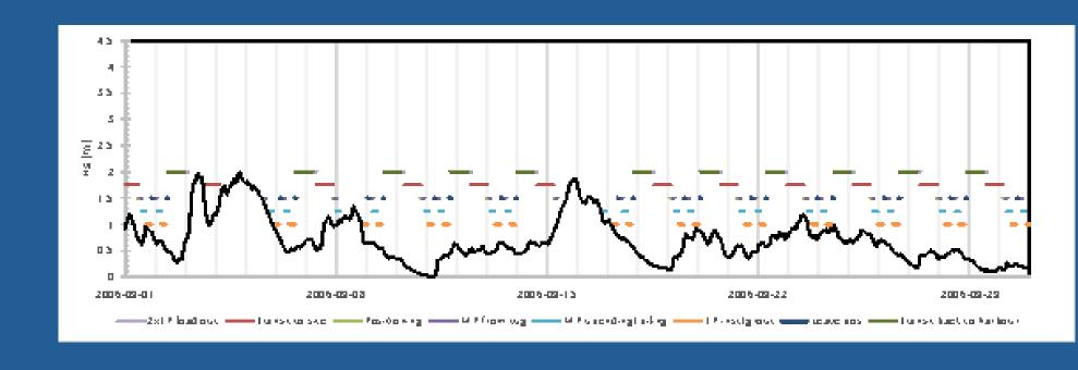
The impact of weather on the Compared to the traditional approach based on weather windows, this newly developed approach provides a detailed picture of the potential number of installation cycles to be executed each month, with a specified degree of certainty (e.g. 80%).
