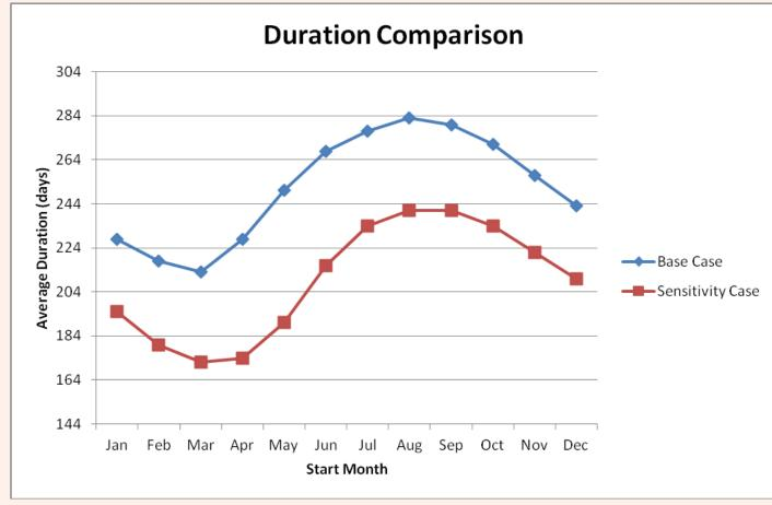
On another project, operations requiring Remotely Operated Vehicles (ROV) were initially assumed to be possible in current speeds of up to 0.8m/s (~1.6knots). Current speeds at the site were strong, with peak spring current speeds frequently reaching 1.5m/s (3knots). The use of ROV operating in current speeds of up to 1.2m/s was showed to significantly reduce the expected installation durations.
