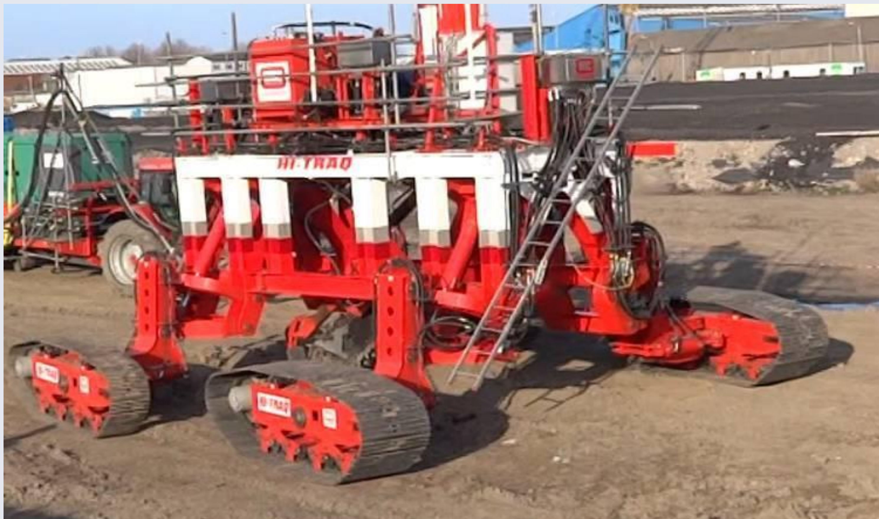
Figure 1. IHC Hi Traq trenching test vehicle
