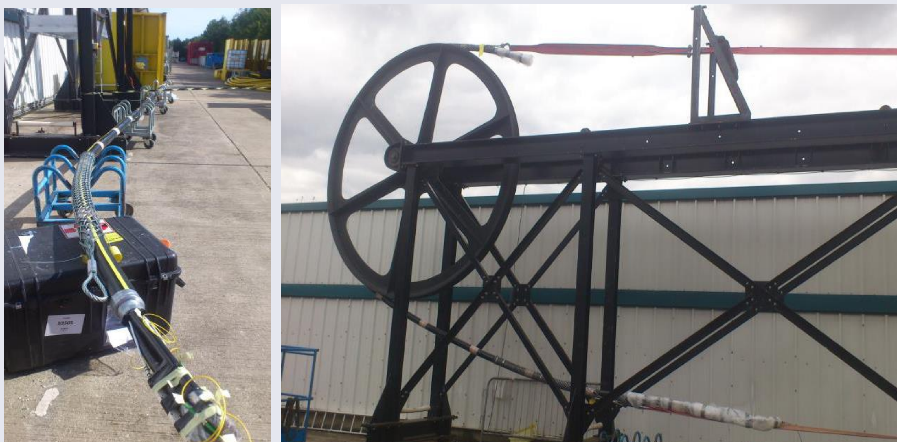
Figure 2. Physical testing process for Smart Cable: combined tension and bending
