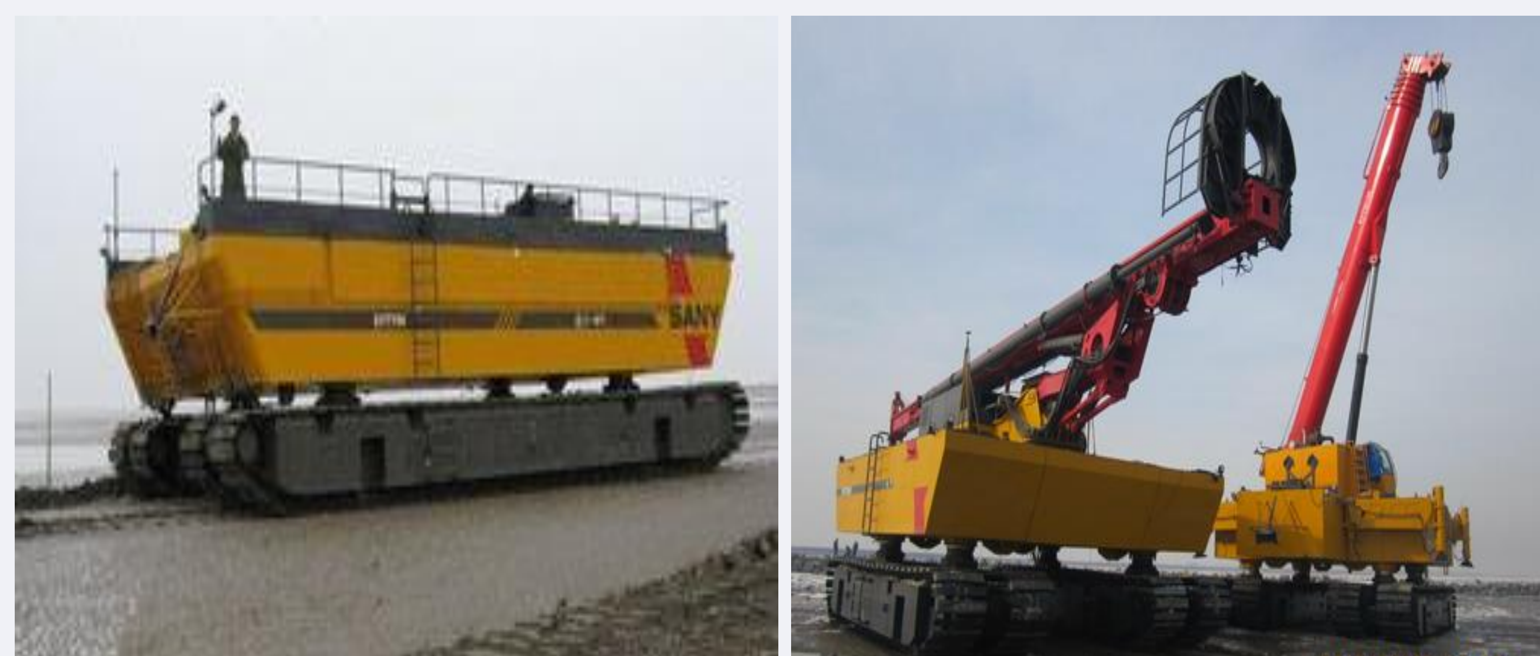
Fig. 2 The installation vessel used for the intertidal area
