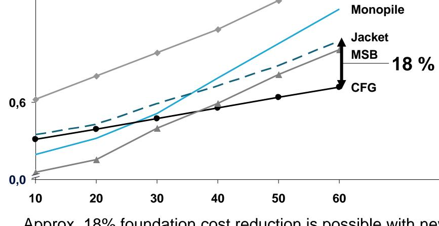
Approx. 18% foundation cost reduction is possible with new foundations at larger depths
