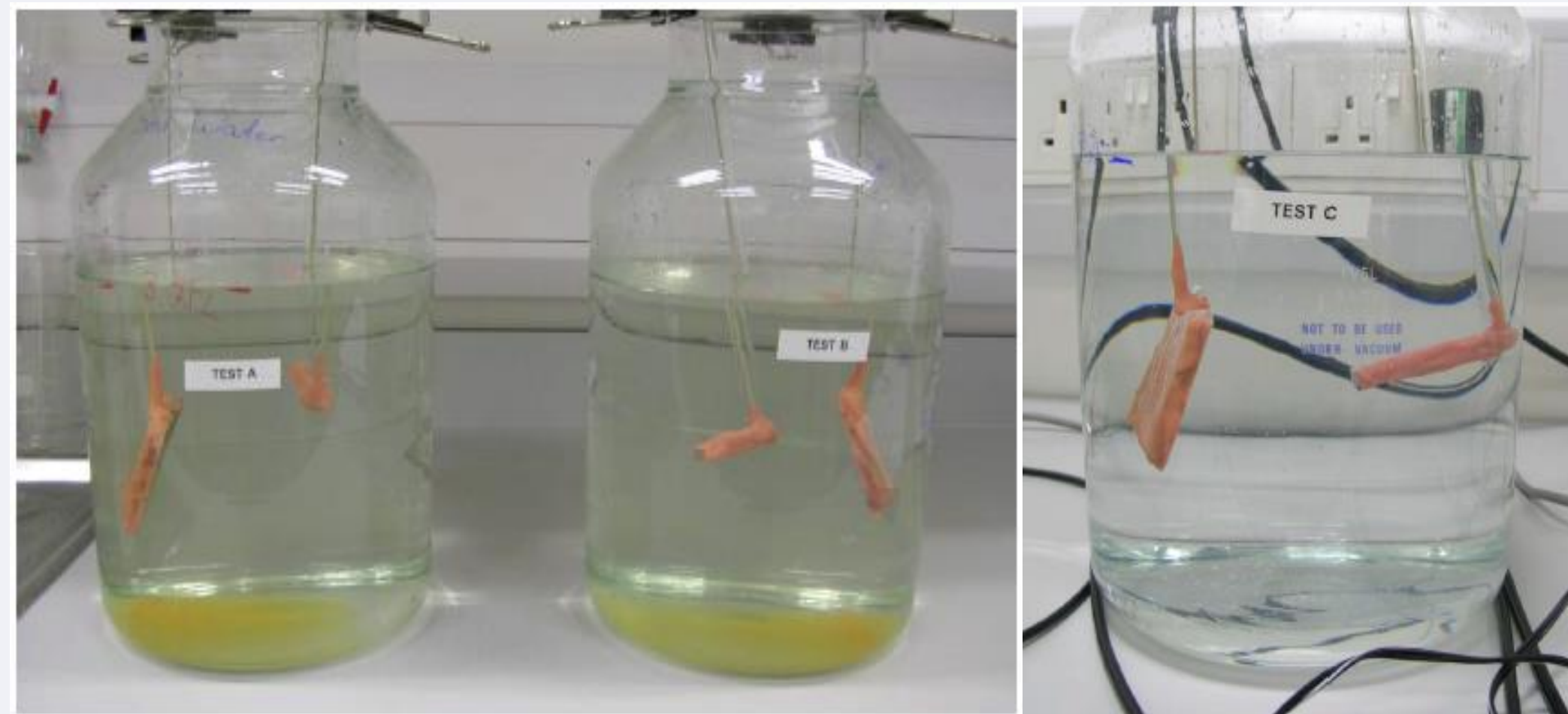
Figure 3 – Laboratory trial 1: Coupled and uncoupled tests (NPL)
