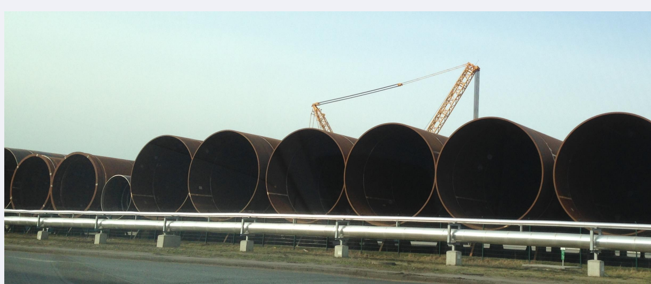
Figure 2 – Monopiles ready for transport – bare steel interior
