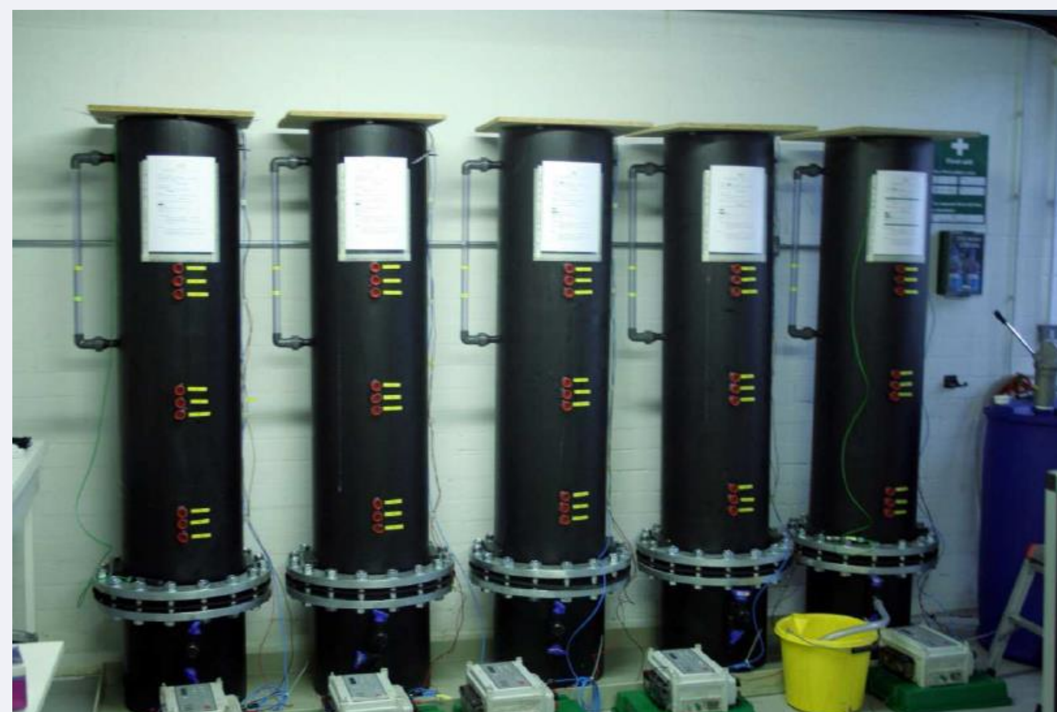
Figure 4– Laboratory trial 2: Zinc and Aluminium anodes with and without gas membrane and with and without tidal replenishment (Intertek)
