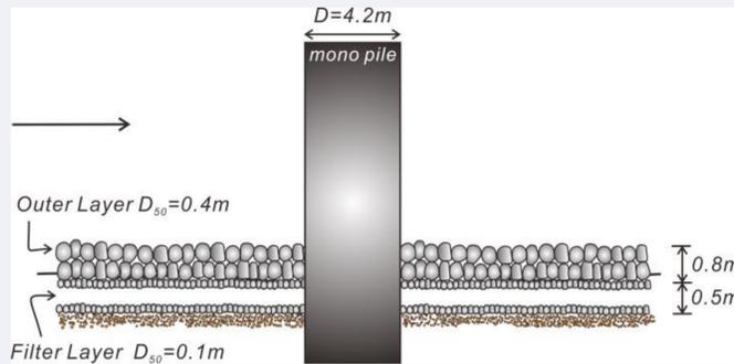
Fig. 1 Schematic sketch of the scouring prevention system of laying finer grade stones as a filter layer under the top scour protection cover
