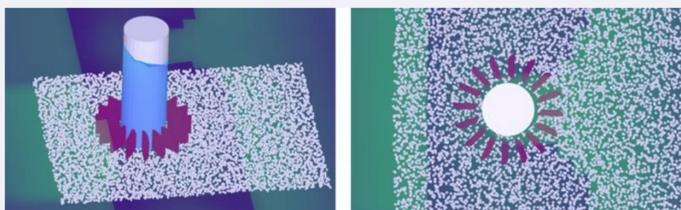
Fig. 7 Plan and side view of the bed morphology after exposure to waves for 80s (hybrid monopile)
