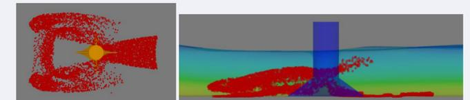
Fig. 6 Plan and side view of the bed morphology after exposure to waves for 80s (quattro-pod monopile)
