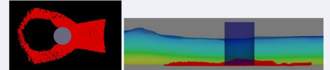
Fig. 5 Plan and side view of the bed morphology after exposure to waves for 80s (simple monopile)
