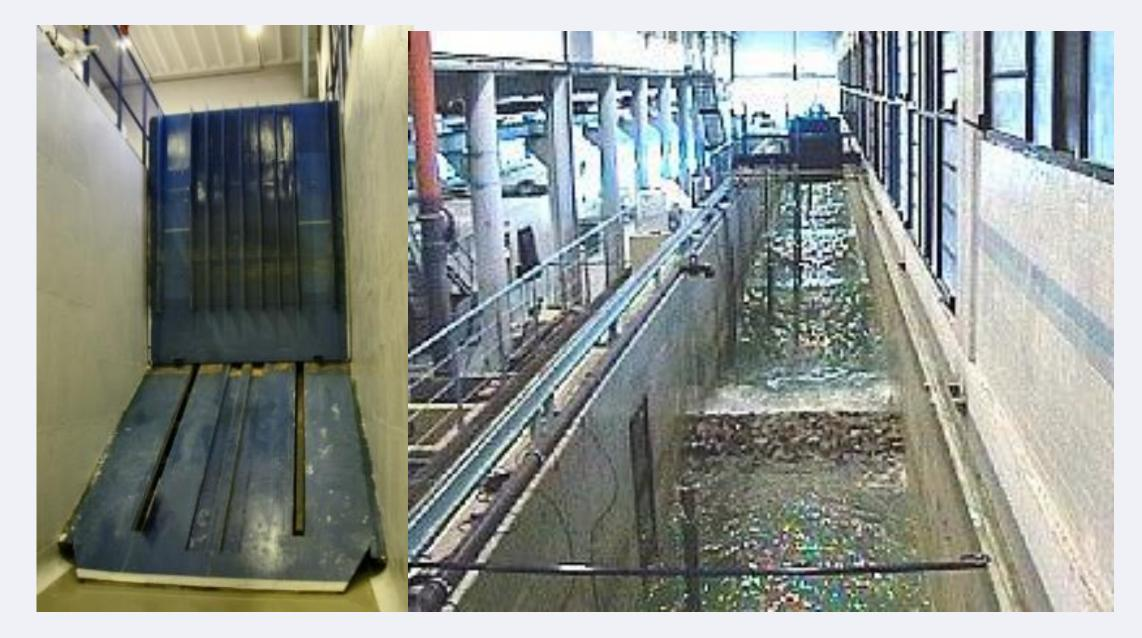
1:100 scale model. The complete experimental campaign included free decay tests, a set of 22 regular wave trains of different periods to determine the RAO's and another set of 21 regular and irregular wave trains in conjunction with a mechanical wind device, simulating the mean thrust force exerted by the wind turbine.
