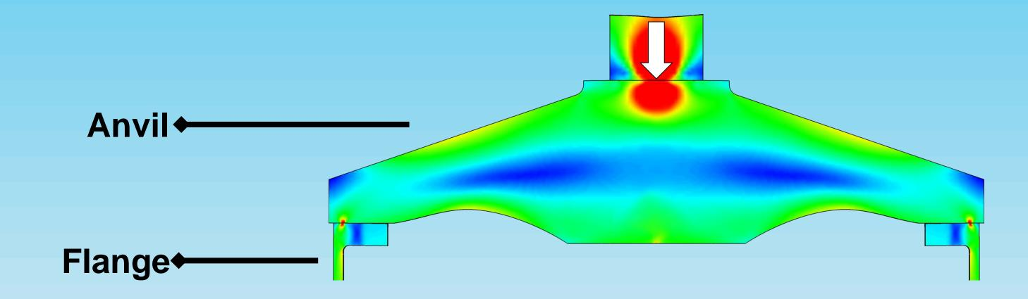
The simple, but acknowledged GRLWEAP soil and hammer model was successfully transferred to a detailed finite element model in LS-DYNA, allowing for comprehensive investigations of pile-driving operations.
