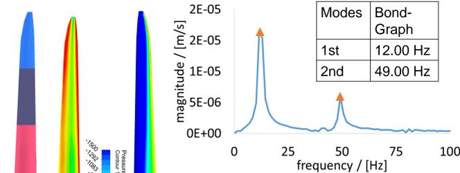
Fig.4. frequency spectrum of high speed shaft translational vibrations due to impact test on hub
