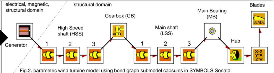
Fig.2. parametric wind turbine model using bond graph submodel capsules in SYMBOLS Sonata
