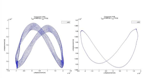
Fig.10. Orbital displacement of power trains and selected components due to gravity load in positive z-direction and eccentricity of hub mass considering torsional vibrations and gyroscopic effects
