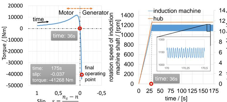
Fig.7. starting behavior of induction machine connected to an electrical network
