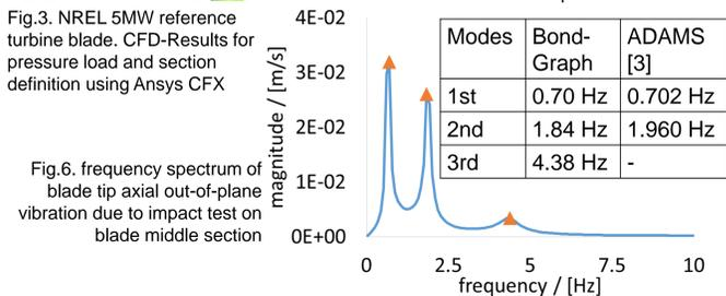
Fig.6. frequency spectrum of blade tip axial out-of-plane vibration due to impact test on blade middle section
