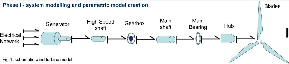
Fig.1. schematic wind turbine model
