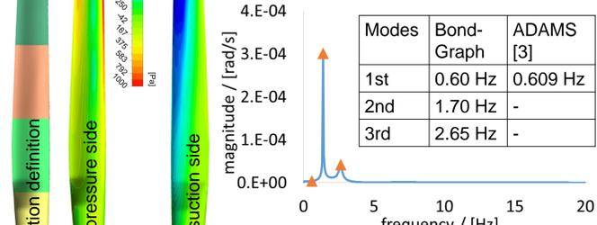
Fig.5. frequency spectrum of high speed shaft torsional vibrations due to impact test on hub
