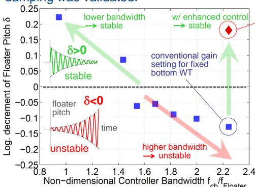
Fig.8 Effect of controller bandwidth on stability
