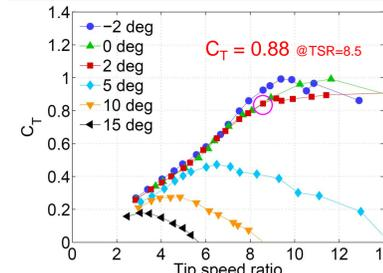
Fig.2 Thrust coefficient
