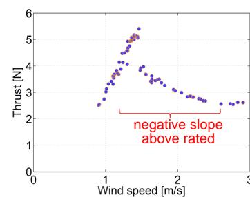
Fig.4 Thrust curve
