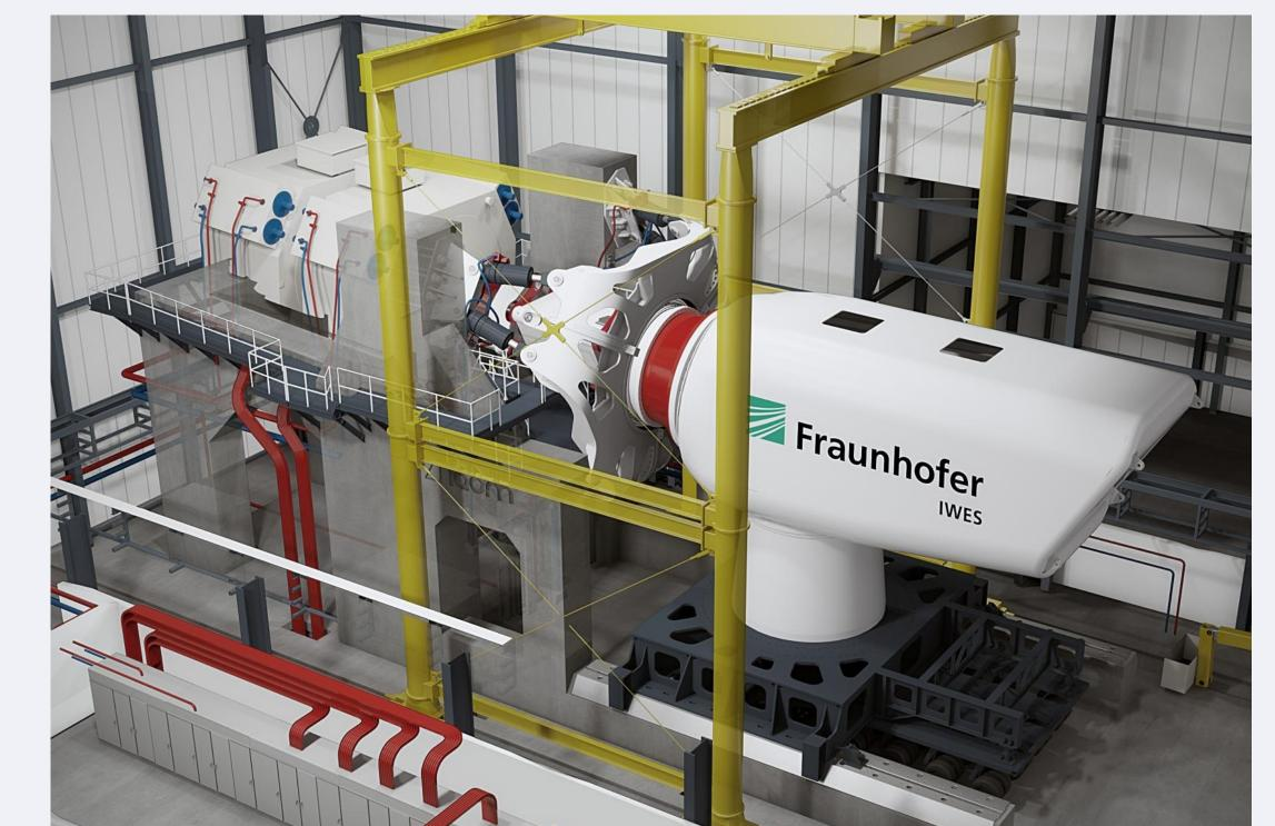
turbines with medium voltage grid emulation and load application system (virtual rotor)
