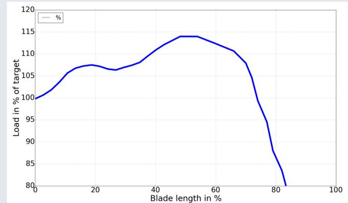
Adding large masses relatively close to the root will increase the load in the root and thereby change the critical point to 70 % of the blade length. The maximum overload is now reduced to 3% at several points from the root to 70 % of the blade length. See also the diagram below:
