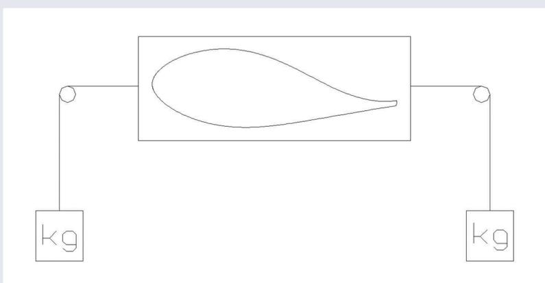
The introduction of masses acting in one direction can be done in several different ways. BLAEST has practical experience with several different methods used both in edgewise and flapwise directions. The above figure shows a method using a wire and a pulley which will add mass in the edgewise direction without affecting the flapwise direction.
