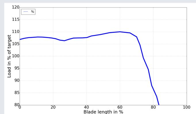
Consequently, it is possible to decrease the overload on much of the blade and at the same time reach the required bending moment at the root. This method will also permit a small increase in the general load level, whereas the overload it kept at an acceptable level. This increase will also permit a reduced number of load cycles. Assuming that the blade is made of polyester, an increase of loads by 7 % will reduce the number of cycles to 50 %.
