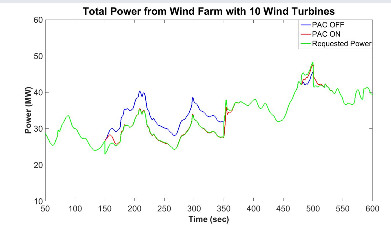
$\succ$  The PAC alters the power output of the turbine by a value  $\Delta P$  [3].
