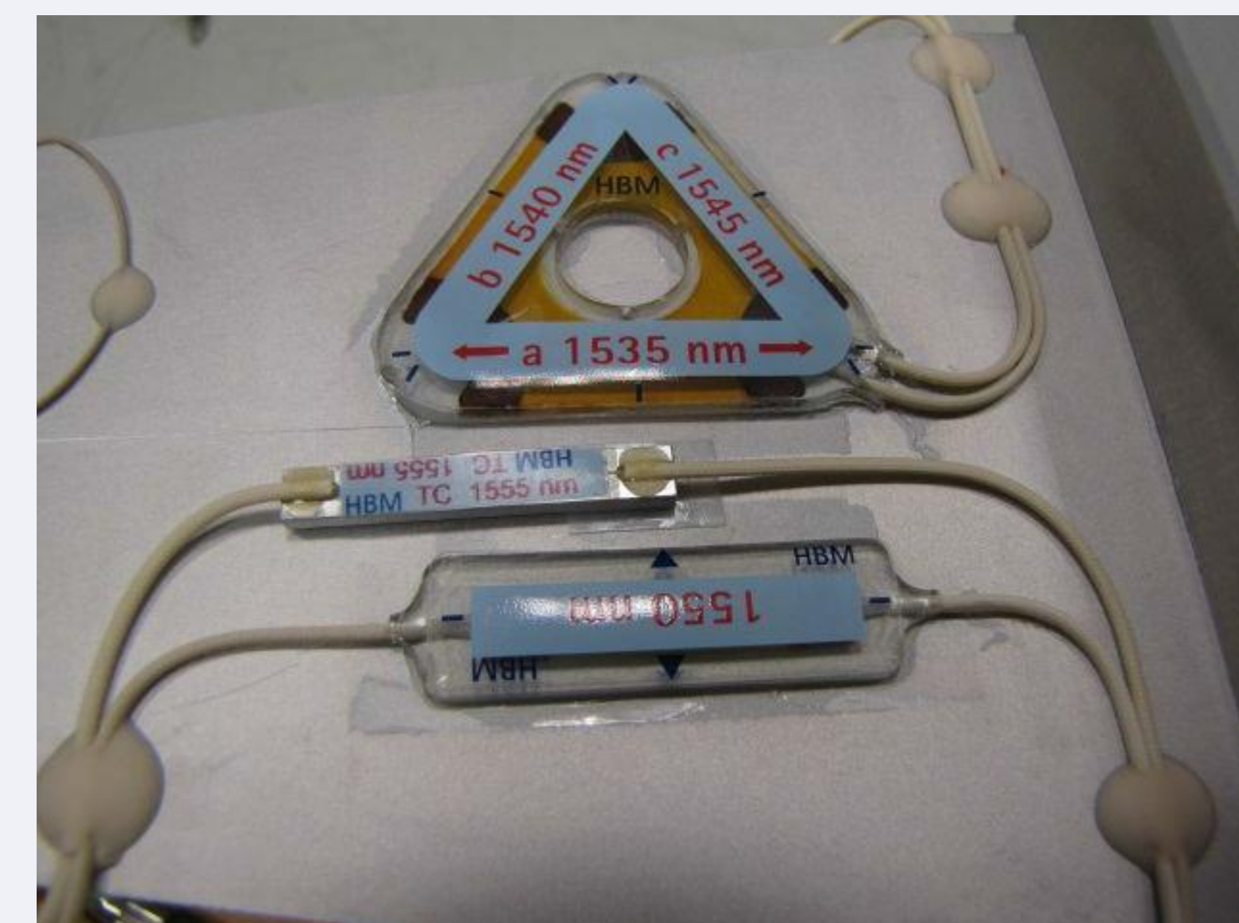
Fig 4: Different types of optical strain gauges >>OptiMet<< by HBM
