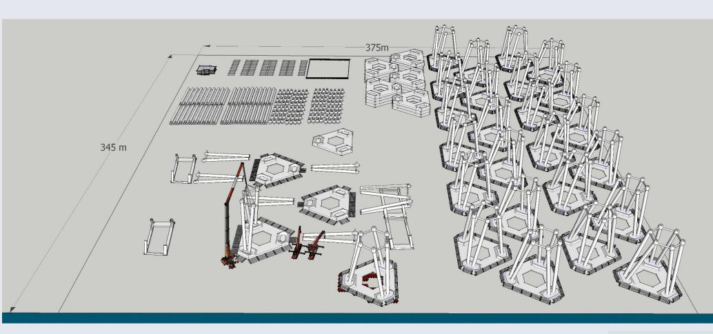
The Gravity Tripod is designed for rapid assembly. As a modular structure manufacturing the components Of Of assembly ahead limits the space and time required to supply a large number of structures.
