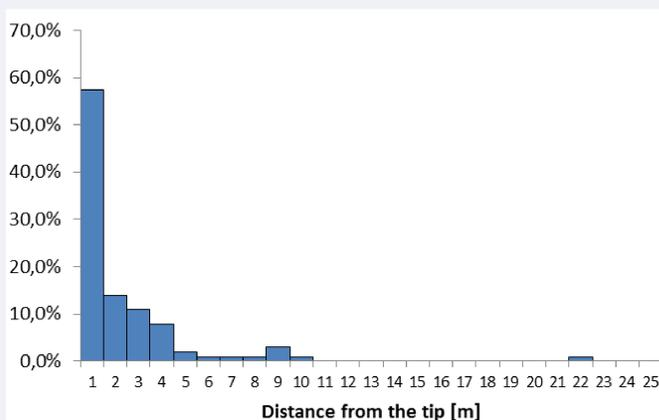
Location of the lightning damage (in percentage) in damaged blades with mixed fiberglass and carbon fibre structure
