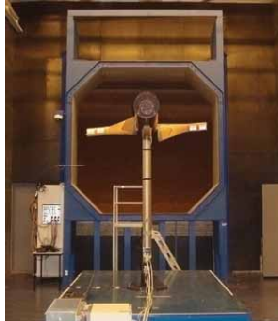
Figure 10: The scale model of a smart rotor in the wind tunnel. The flaps are the silver area’s in the outboard section of the blade.
