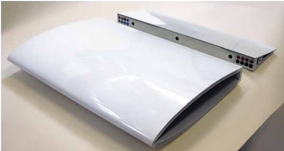
Figure 9: Demonstrator of a blade section with a R-phase SMA activated trailing edge
