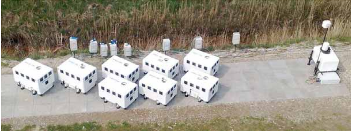
Figure 32: Commercial LIDARs undergoing test at Høvsøre, Denmark. UpWind has contributed significantly to wind LIDAR development and testing.
