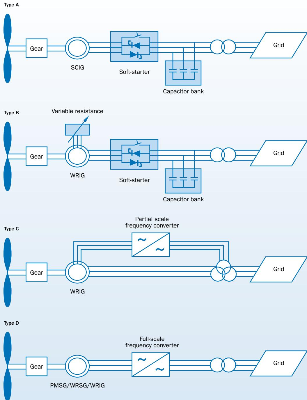
SCIG = squirrel cage induction generator; WRIG = wound rotor induction generator; PMSG = permanent magnet synchronous generator; WRSG = wound rotor synchronous generator
