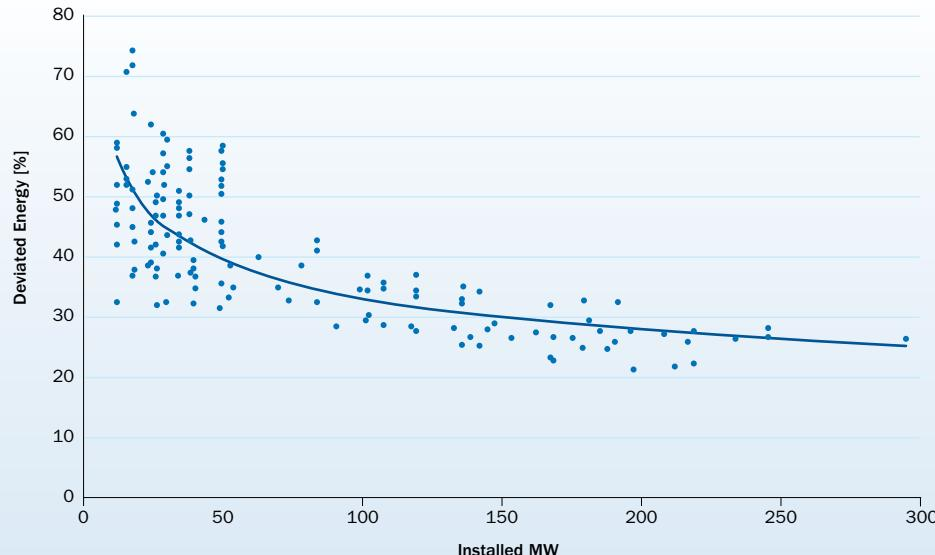
The aggregation of wind farms reduces the mean absolute percentage error (MAPE) from 40% to approximately 25% of deviated energy.
