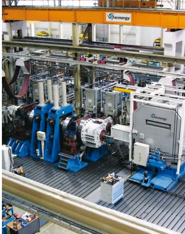
7.5 MW test bench at Winergy gearbox factory
