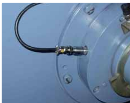
The CMS sensor for the high-speed shaft of the generator
