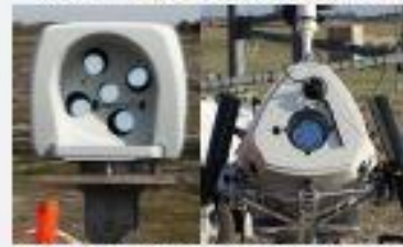
Pictures of the 5-beam Demonstrator (left) and the Zephir Dual Mode (right), during their calibration at DTU Wind Energy test site, Høvsøre, DK
