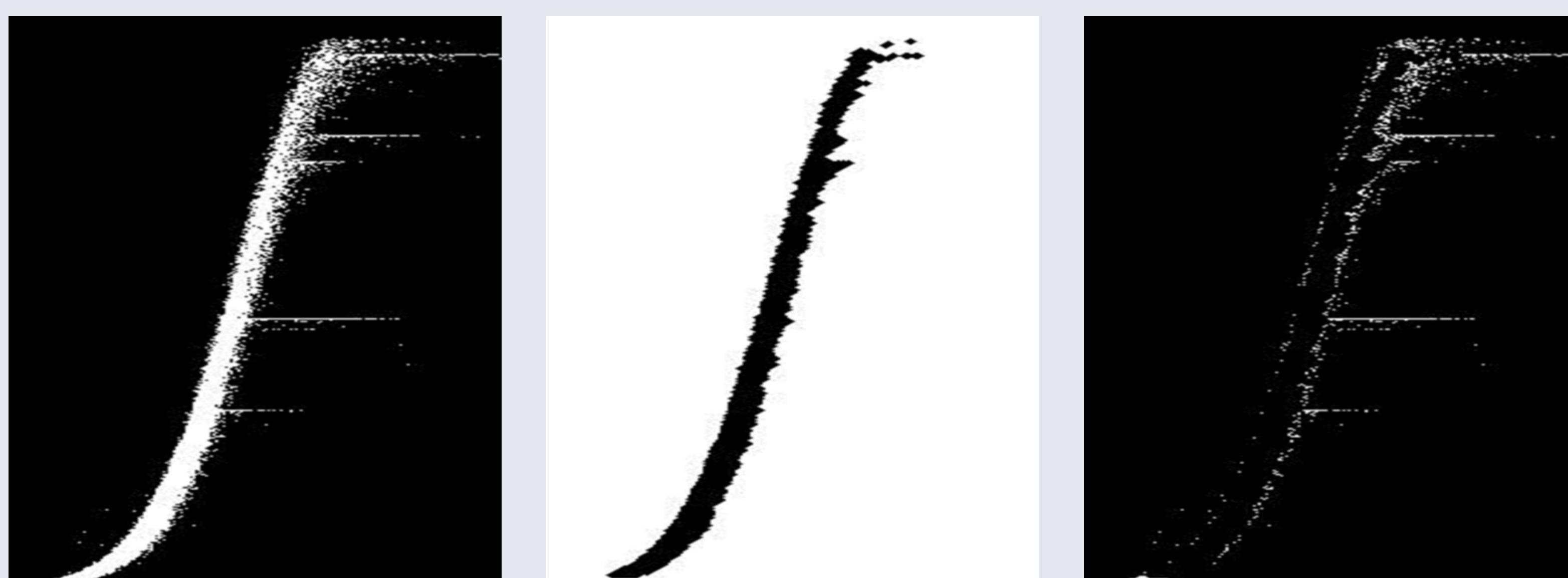
Figure 2 : Image processing of power curves (left: binary version, centre: mask, filtered power curve)
