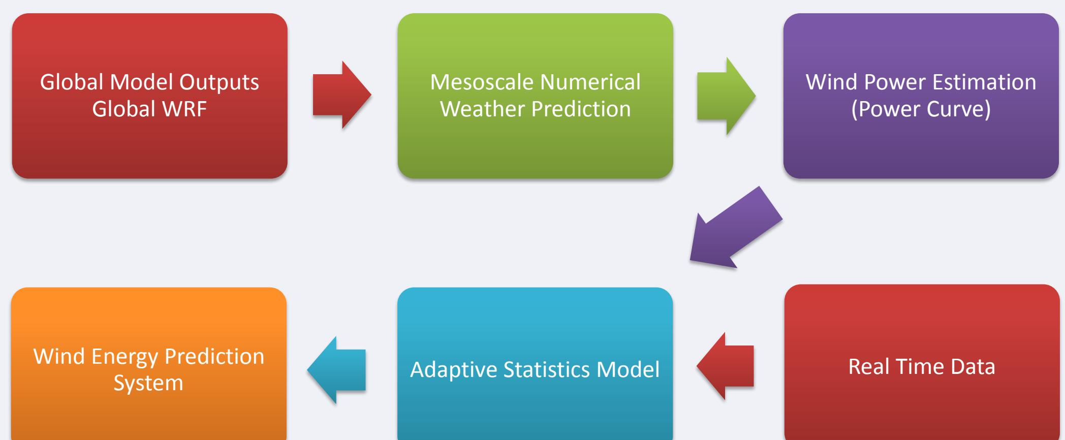
Figure 1. Short term Wind Energy Prediction System (SWEPS)
