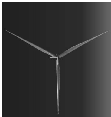
Figure 2: Three-bladed rotor model used in CFD.
