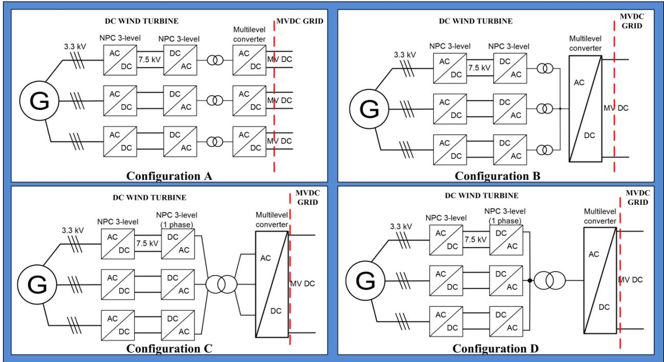
Figure 1: DC/DC converter configurations for a multi-phase generator system.
