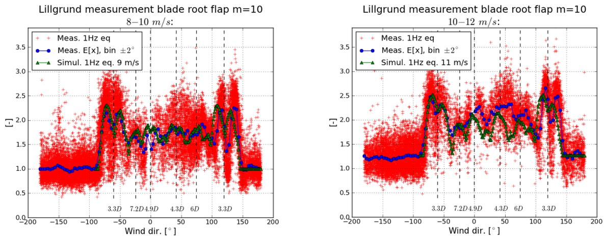
**Figure 2:** Measured and predicted blade flap fatigue equivalent polar. a) 8-10m/s; b) 10-12m/s.
