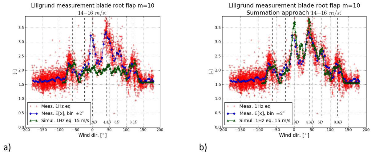
**Figure 3:** Measured and predicted blade flap fatigue equivalent polar. a) Old<sup>4</sup> DWM version; b) revised DWM version.
