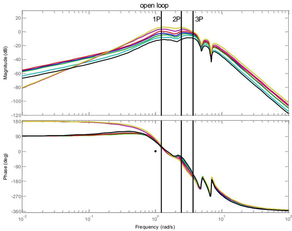
Figure 5: Open loop Bode diagram for IBC2
