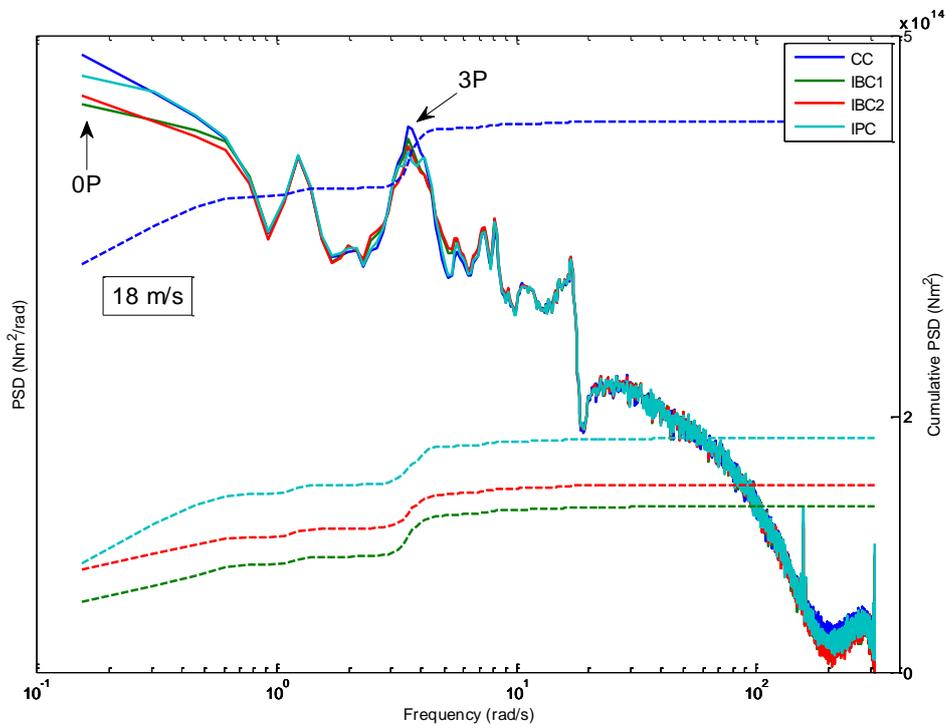
Figure 7: Power spectra comparison for fixed hub My between different controllers
