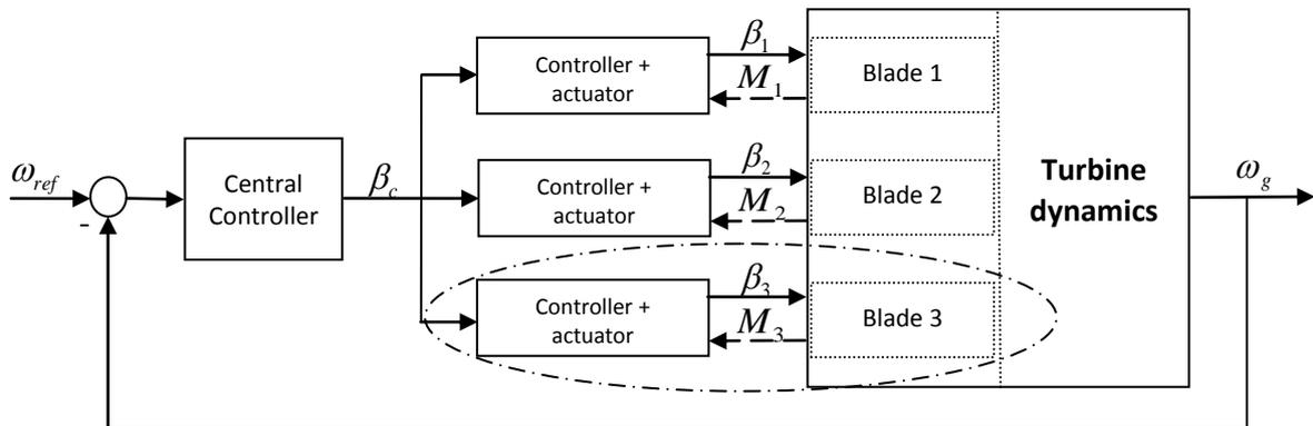
Figure 3: IBC based on single blade model
