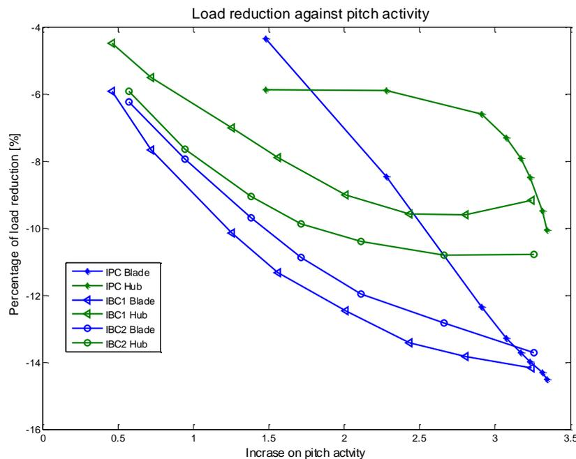
Figure 8: Load reduction against pitch activity for IBC1, IBC2 and IPC
