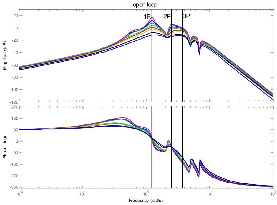
Figure 4: Open loop Bode diagram for IBC1
