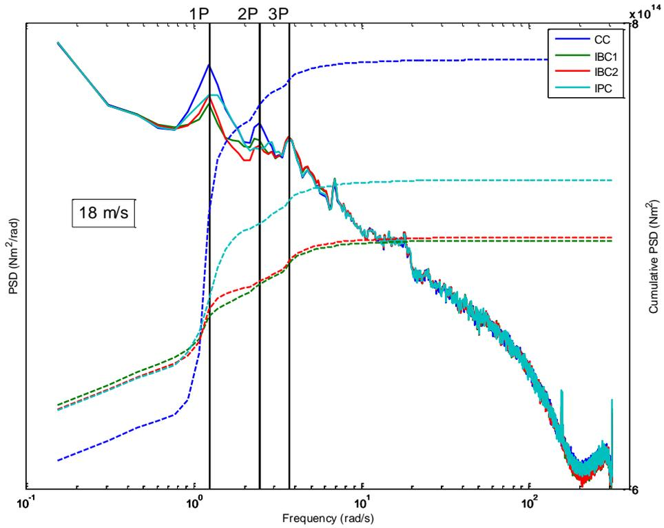
Figure 6: Power spectra comparison of blade root My for different controllers
