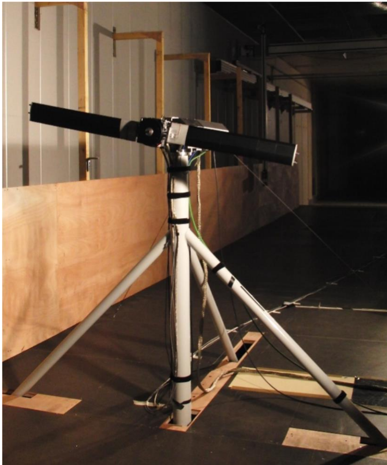
Figure 3: 2-blade wind turbine bench.
