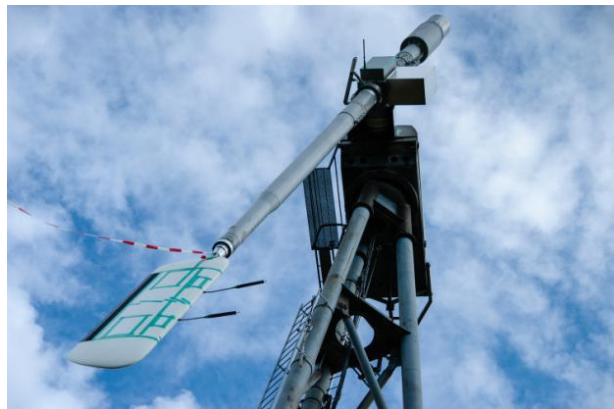
Figure 4 The photo to the left shows installation of the boom with the blade section in June 2014. On the photo to the right the blade section with the flap (black colour) can be seen as well as the two five hole pitot tubes.
