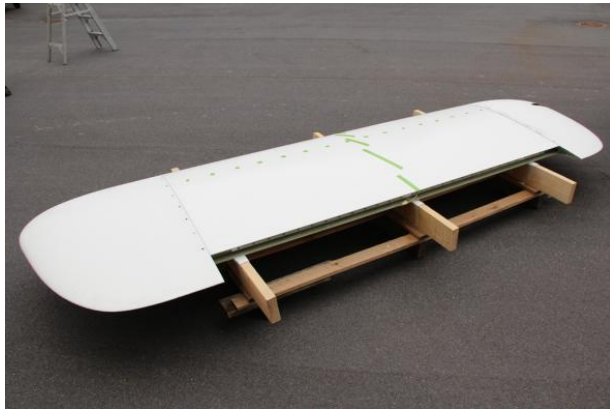
Figure 3 To the left is shown the 2x1m blade section + end caps before mounting the 2m long flap. To the right a sketch of the rotating test rig.
