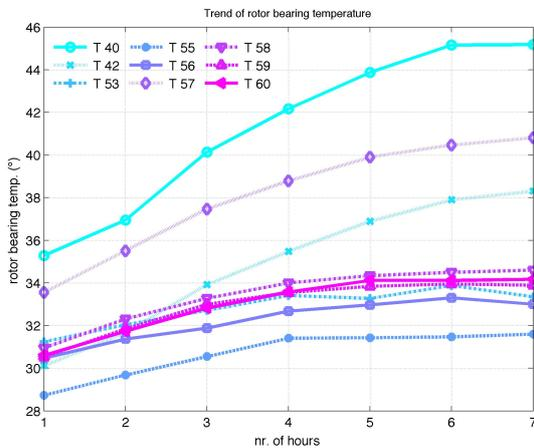
**Figure 7.** Time evolution of rotor bearing temperature after turbine reboot.
