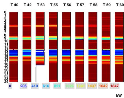
**Figure 5.** Graphical map: fault occurrence. Active power in background.
