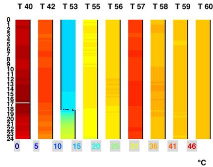
**Figure 6.** Graphical map: intense wind speed. Rotor bearing temperature in background.
