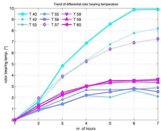
**Figure 8.** Time evolution of rotor bearing temperature after turbine reboot: difference against reference value at machine stopped.
